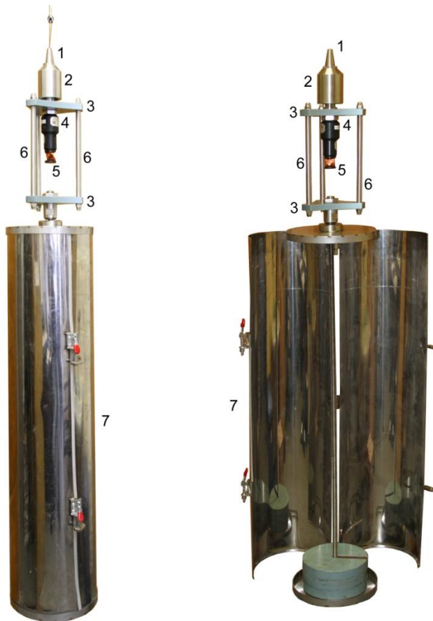
Fig. 27 Suspension for an omnidirectional prism coaxially inserted above the plummet
