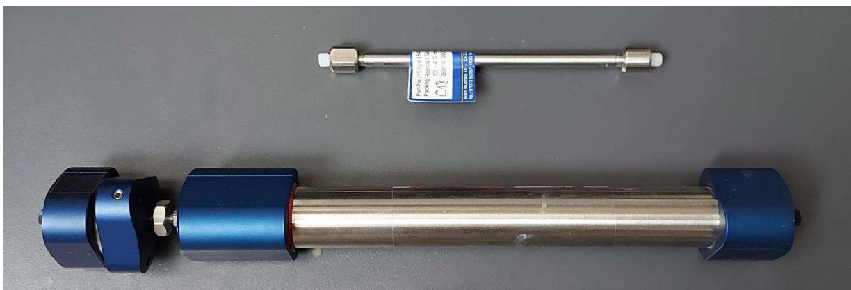
Figure 1. Analytic (top) and preparative (bottom) HPLC columns
